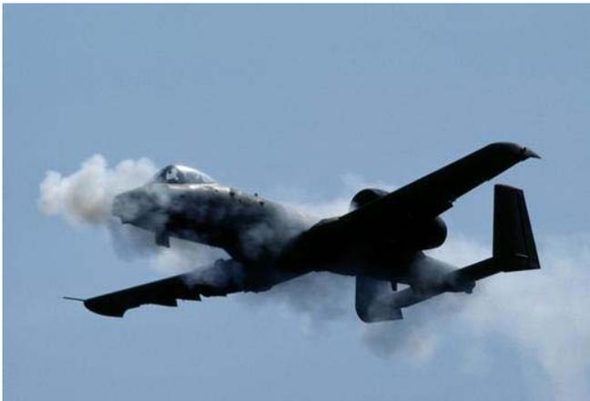
**This A-10 Warthog Was Designed For A Very Specific Purpose - Tank Busting. As a result, it does this very well, flying low and slow while firing depleted uranium rounds (shown) from the cannon that the entire aircraft was designed and built around. It was a star in the**
